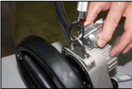
Step 1 - Align the ladder bracket adapter with the anchorage ring/carabiner and insert.
