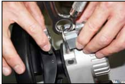
Step 2 - Place the adapter plate on the opposite side of the anchorage ring.
